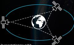
In geostationary orbit, three satellites can provide continuous global coverage (excluding the poles) 1.5 billion km
